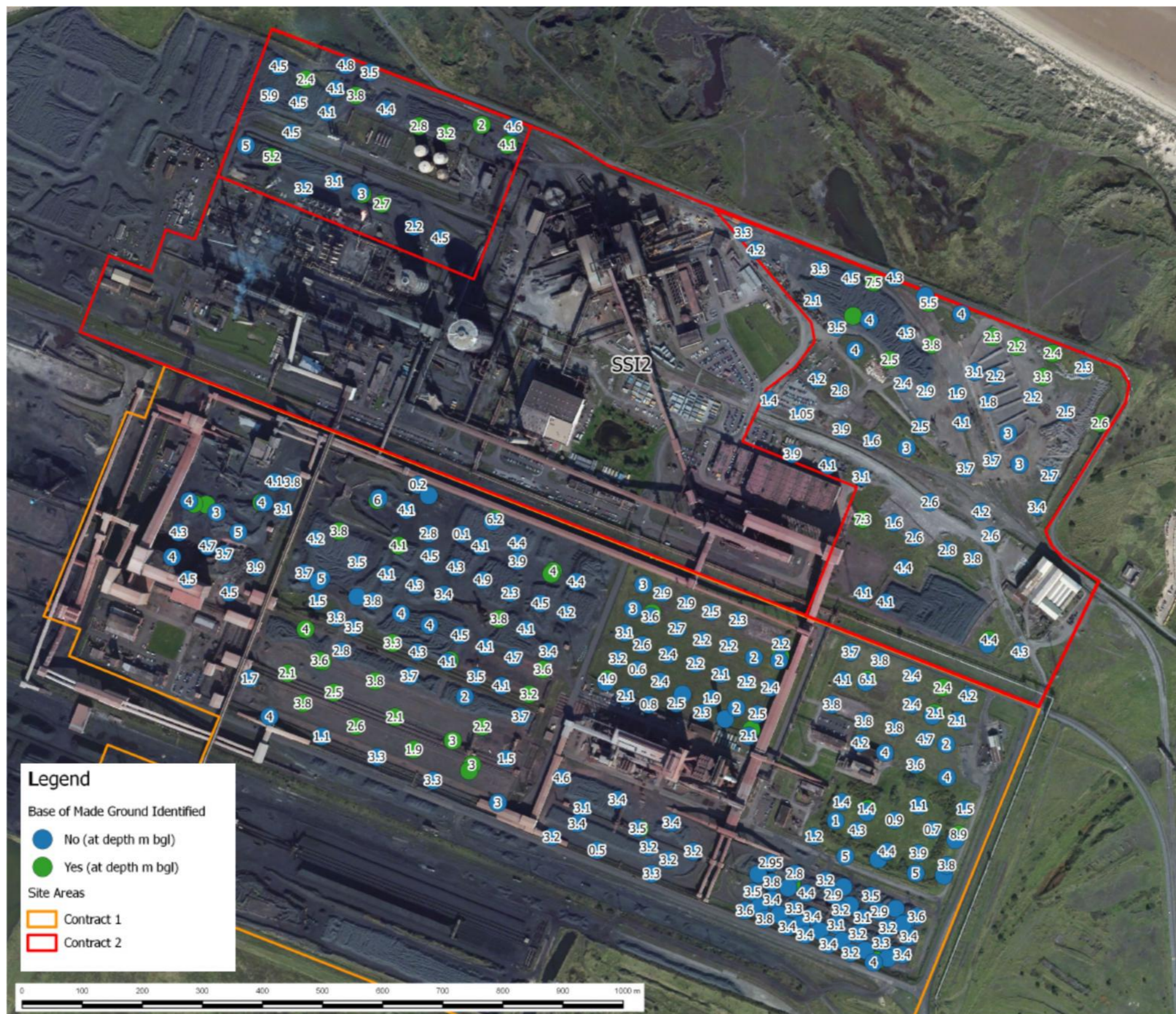
SSI3A Figure 3 – Depth of Made Ground Encountered
